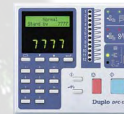
10-key control panel with LCD window displays current operation status/mode and allows for full control of the entire system.
